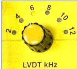
This switch allows selecting the excitation frequency of the primary coil of the LVDT transducer. The frequency depends on the layout of the transducer as defined by its manufacturer. The Feedback-Expert electronic enables to set the frequency from 2 to 12 kHz in steps of 2 kHz. The selected frequency will be shown by a LED display.
