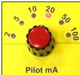
This switch allows setting the current of the pilot servovalve. The current ranges are from 0 to 2 mA, 0 to 5 mA etc. and the current will be controlled by the ValveExpert test rig and this with the voltage range from  $\pm 10$  Volt. Attention: the current range goes into the loop gain; a too high current range may cause instabilities.
