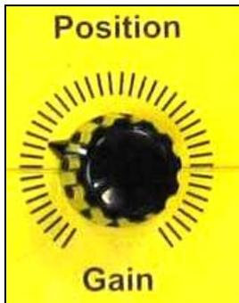
This potentiometer allows adjusting the range of the position output signal. The adjustment is usually done for the maximum stroke of the spool and a correspondent voltage will be adjusted (for example 10 Volt)
