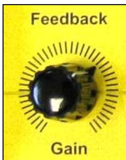
This potentiometer allows adjusting the loop gain of the spool position control. This adjustment has to be done carefully. A too high loop gain will cause instabilities. A too low loop gain will influence the test results of the transducer output (Hysteresis, non linearity...)
