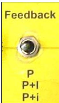
The servo-amplifier is either a proportional or proportional-integral amplifier, and the markings mean:
