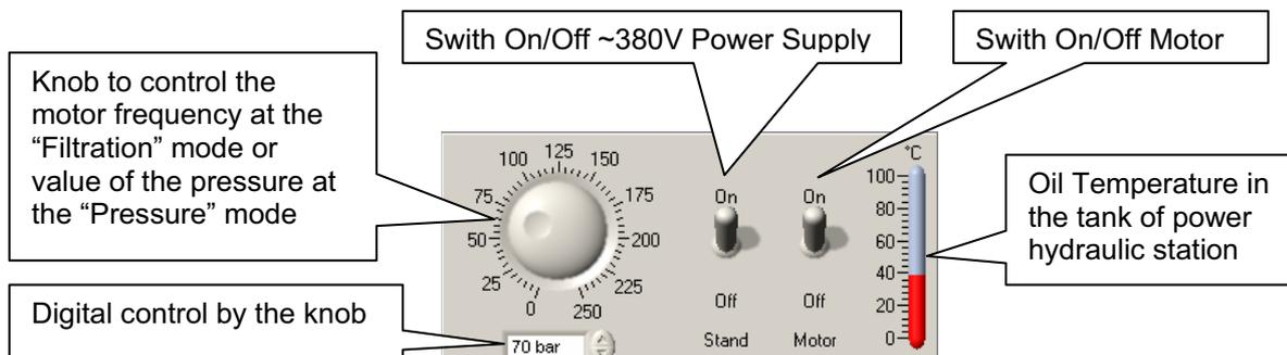
**Picture 21.** The main hydraulic station controls. Note that you are not able to switch the motor until ~380V is not switched on. Note also that high temperature will immediately stop the motor.
