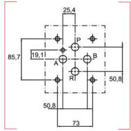
Norm ISO 10372-06-05-0-92 This corresponds to the basic port pattern on which can be mounted additional adapter manifolds. The base port pattern is compatible for following servovalves: MOOG X072, MTS 252,3x, STAR 8XX ULTRA 4550 (with internal pilot)
