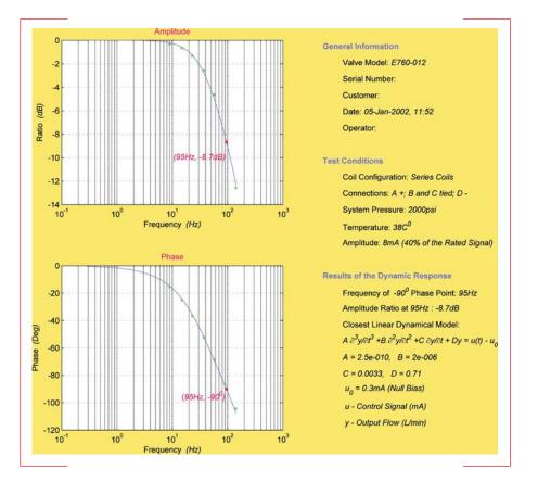
The results of the dynamic tests are imprinted as a Bode diagram as is common for servovalve manufacturers. The green points in the diagram show the actual measured values. The blue line represents the evaluation of the differential equation which best represents the dynamics of this valve.
