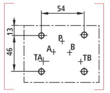
Norm ISO 4401-05-05-0-94 Norm NG10 For following servovalves : MOOG D634 MOOG D661 REXROTH 4WRAE REXROTH 4WRDE REXROTH 4WREE REXROTH 4WREE REXROTH 4WRKE REXROTH 4WRSE REXROTH 4WRSE REXROTH 4WRSE REXROTH 4WRSE REXROTH 4WRZE STAR 1652R
