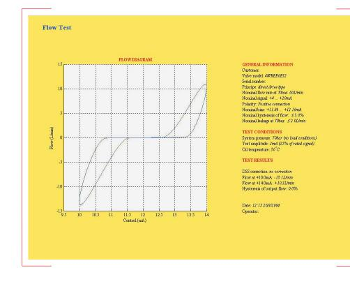
This diagram shows the flow curve of a REXROTH proportional valve. This valve is equipped with a ramp function. The ramp objective is to slow down the command signal of the valve, which therefore has an intentionally slower dynamic response. As can be seen, the curve is "blown up" and it is difficult to recognize the hysteresis, the overlap or the curvilinear form of the valve. (The curve was sampled with a control signal of 25% of the nominal signal and a frequency of 0,01 Hz.)
