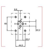
Norm ISO 10372-04-04-0-092 For following servovalves : ATCHLEY 209, MOOG X062, MOOG X073, MOOG X076, MOOG X760, MOOG X761, MOOG X765, MTS 252.2x, PEGASUS 122A REXROTH 4WSE2EM10A-45 STAR 5XX ULTRA 4653, VICKERSS M4-20, VOSKHOD UG176 (with internal pilot)
