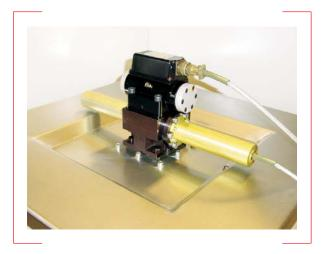
To evaluate the dynamic performances of a mechanical feedback servovalve, a frequency response piston has to be mounted below the valve being tested. The piston is equipped with a position transducer which allows controlling the piston in its mid-position and a velocity transducer for the flow measurement. For electric feedback valves such a frequency response piston is not necessary as the signal of the spool position can be used for the dynamic evaluation.
