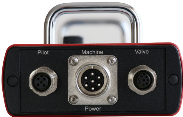
Figure 8: Connector view of the test device ValveExpert Checker 2.4. See Tables 3 and 4 for Pin assignment.
