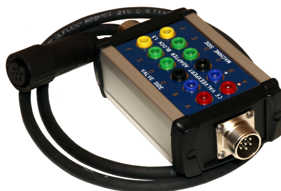
Figure 13: ValveExpert Adapter 1.5 allows to check all the signals with an external multimeter or oscilloscope (not included by default). The adapter contains also LED indications of the positive and negative power supply.
