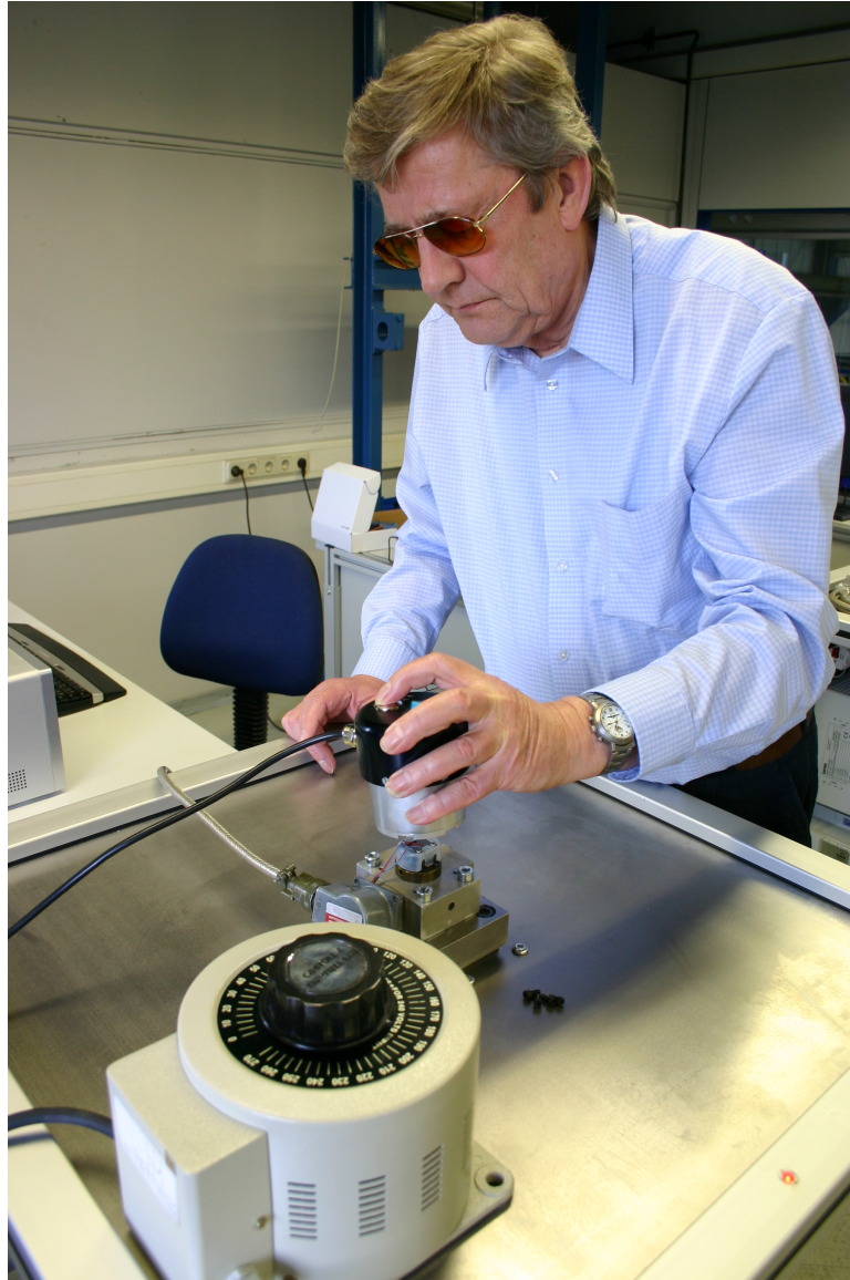
Figure 1: Magnetizing of a Moog servovalve
