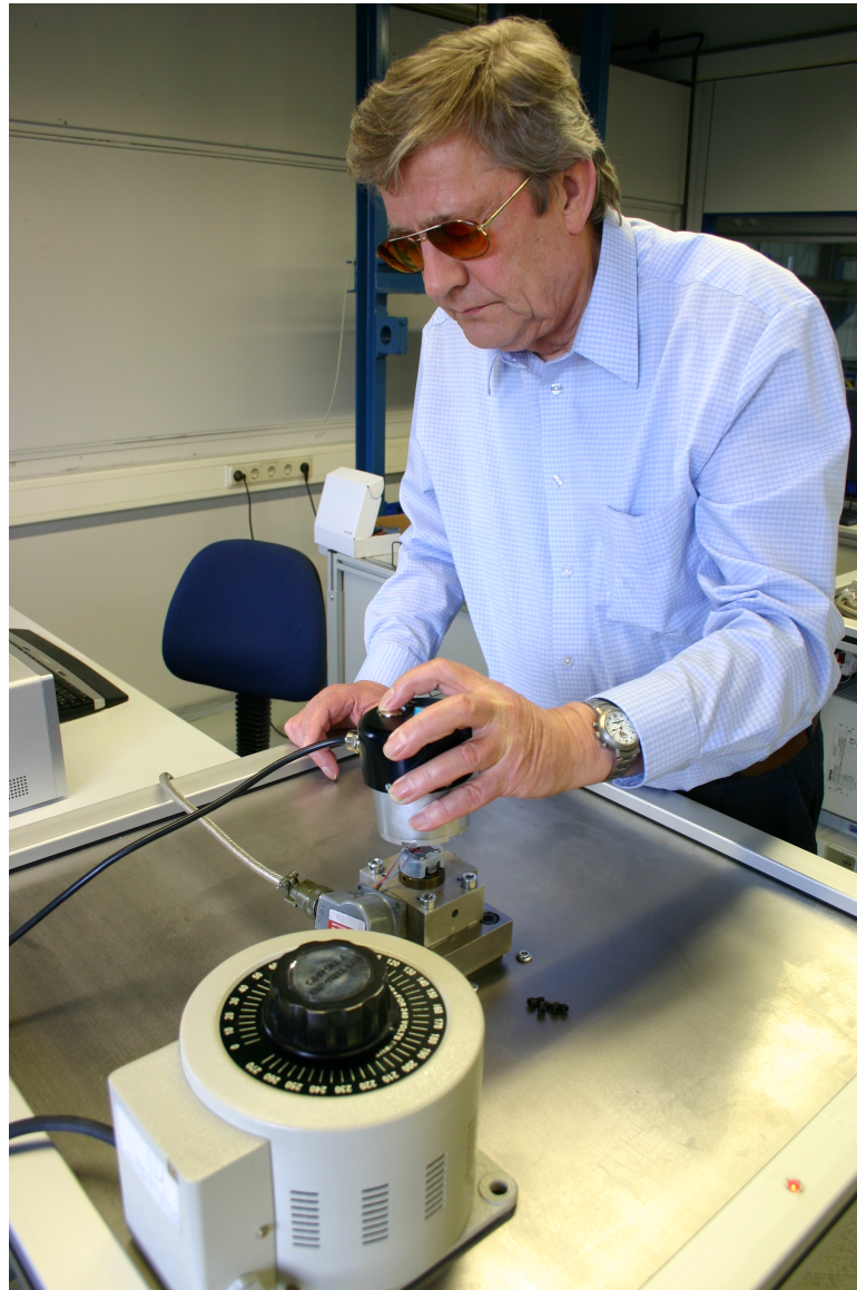
Figure 2: Magnetizing of a Moog servovalve
